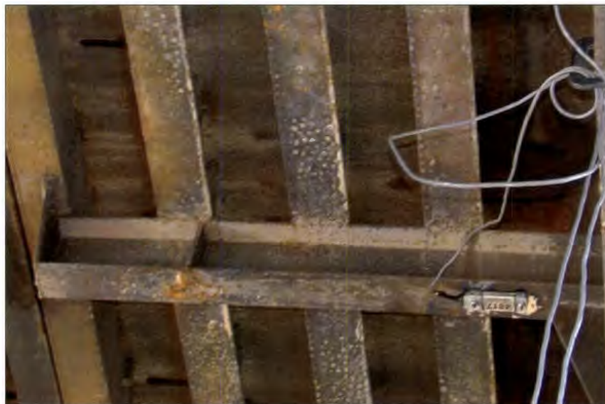
b. Strain transducer 11 on an S-shaped transverse member
