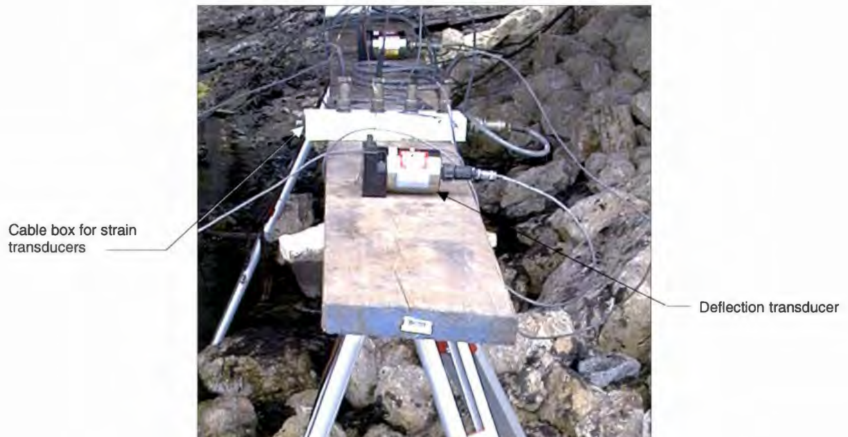
b. Deflection transducer for the exterior girder at the 1/4 span
