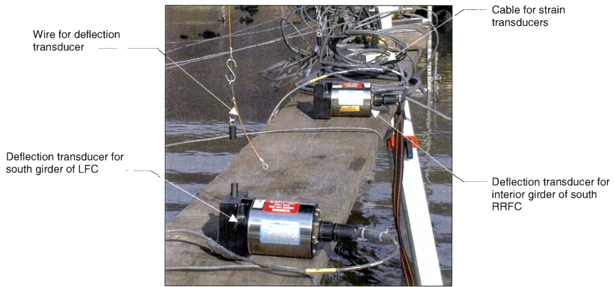
Figure 3.8. Deflection transducers used on DCB.
