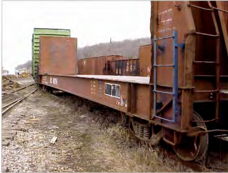
a. The 56-ft V-deck RRFC prior to trimming
